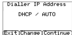
If you are using a DHCP network connection, click «Continue». If the customer has requested that a fixed IP address is assigned, then click «Change».
