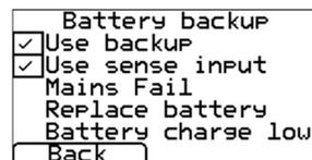
This screen also shows faults with the battery backup (main fail, batteries need replacing or low battery charge), if present
