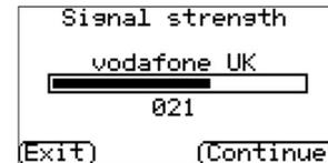
If the signal strength is below or close to minimum then try to reposition the antenna or use an external high gain antenna to improve signal strength (if necessary). Re-run the signal strength test and reposition again if necessary to gain best signal strength possible.
