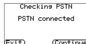
If PSTN is not connected, please check the cable and connection to the PSTN line. After reconnecting, it can take up to 30 seconds to detect.
