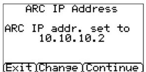
**Note:** Only the primary/main ARC IP address needs to be entered on the terminal, all backup or alternative IP addresses are downloaded from the ARC to the terminal on the first polling communication.
