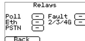
Click on the relevant box for the relay to be used for indicating this failure.
