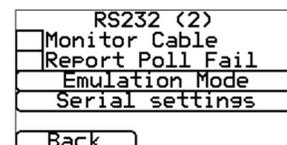
For this to work, the ARC must enable the “serial port monitoring” on the ISA receiver software in order to receive alarm notifications on this status.
