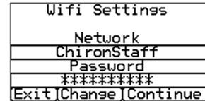
You can then change the parameters required, such as network SSID and access password.
