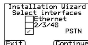
For single path communications, the terminal can use Ethernet, Wi-Fi or cellular paths. For dual path communications, select cellular and one of the other paths.
