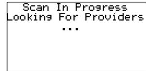
For a reliable cellular connection, there should be at least two base stations with signal strength (CSQ) of ten or more for the network to be used. If the signal strength is below that, try to reposition the antenna or the terminal or swap the current antenna for a high gain antenna. Then run the network scan again to check signal strength.
